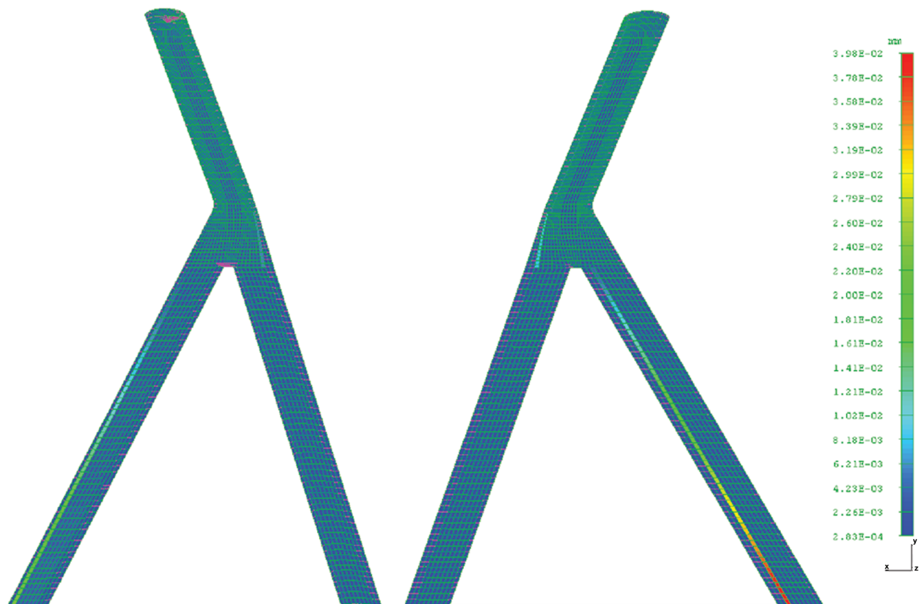
Fig. 11 Top view (left) and bottom view (right) of material distribution for 0 deg ply orientation on the lowest observed (second optimal) configuration.
